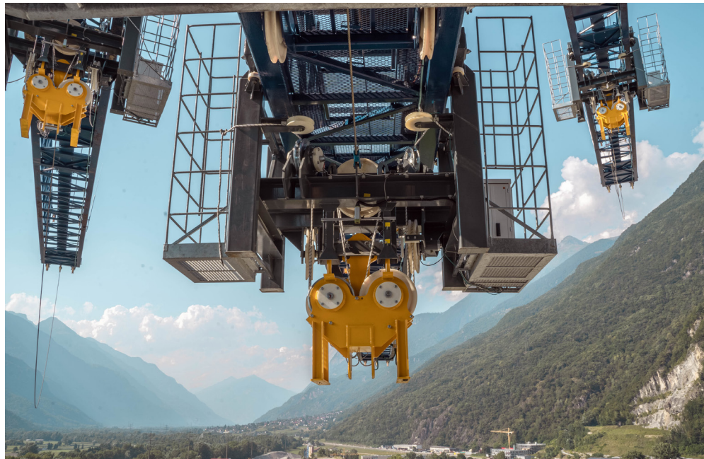
Above: The crane stands 80m over a valley in Ticino, Switzerland. The concept is scalable to a 100m-high tower using up to 8,000 blocks
